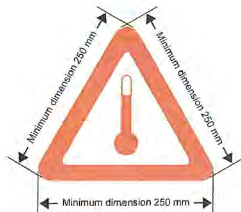
Mark for carriage at elevated temperature
