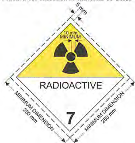
Placard for radioactive material of Class 7
