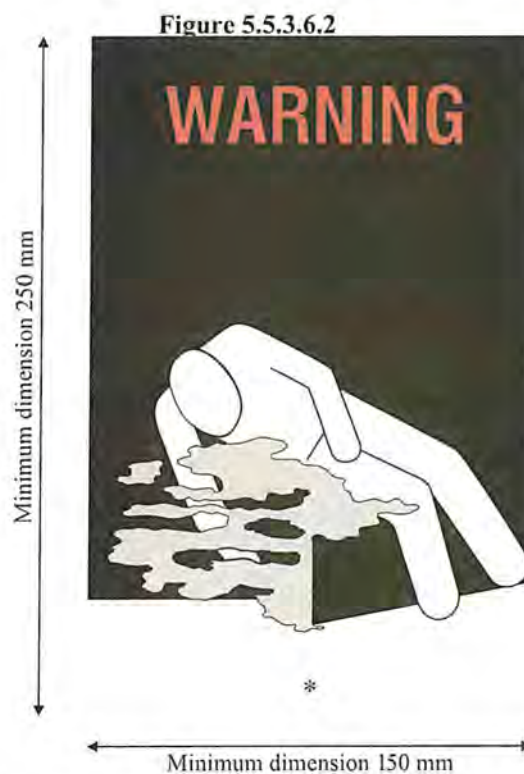
Asphyxiation warning mark for vehicles, wagons and containers
